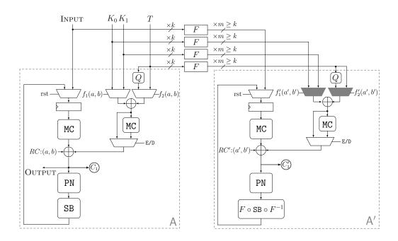
**Figure 11:** Round-based design architecture of CRAFT with fault detection,  $m \ge k$  (control unit not shown, checking PN output not required).
