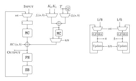
Figure 8: Round-based design architecture of CRAFT supporting tweak, encryption and decryption
