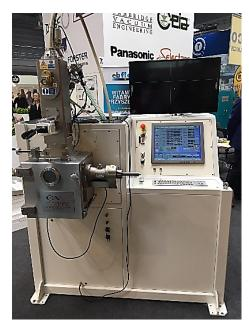
FIGURE 6. CVE – EBW welding source 60 kV.
