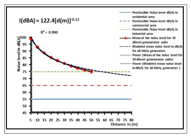
Fig. (2): Comparing of the mean noise level in dB(A) for all thirty generator sites as a function of distance with the permissible noise level s in dB(A) for residential, commercial, and industrial areas.
