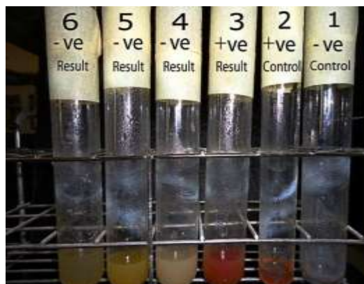
Figure (1) shows the result of qualitative determination of Fumagillin in honey samples. 1- negative control (acetone, sodium thiosulfate, and phenolphthalein) ,2-Positive control(fumagillin , acetone, sodium thiosulfate, and phenolphthalein) ,3- Positive result, red color (sample contaminated with fumagillin),4,5 and 6- negative results (sample non contaminated with fumagillin).
