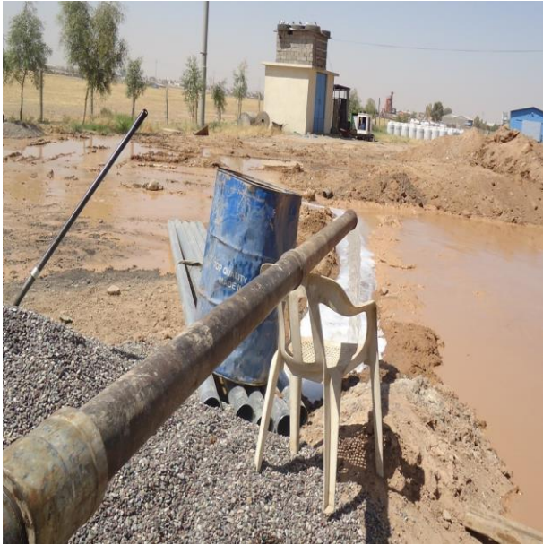
Figure 2 measuring discharge during pumping test
