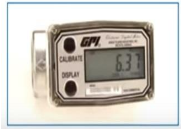
Figure 2 measuring discharge during pumping test
