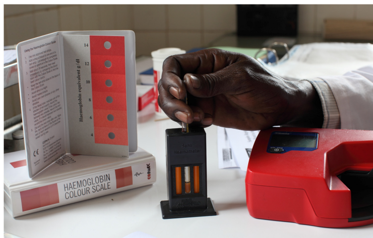
Figure 1. The Haemoglobin Colour Scale, Sahli's meter and HemoCue® analyser for rapid assessment of haemoglobin status.
