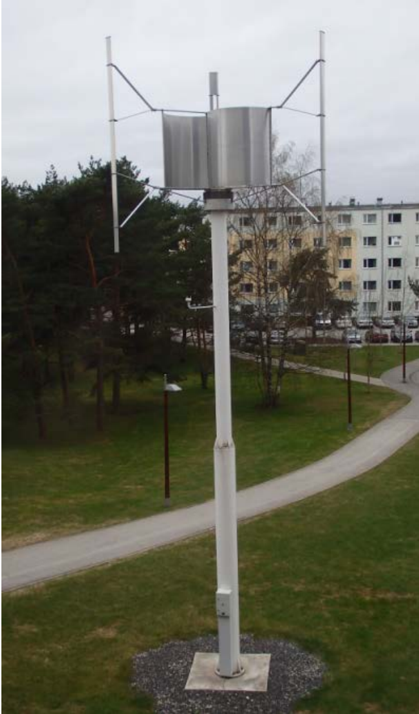
Fig. 15: Prototype generator installed into vertical axis wind turbine.
