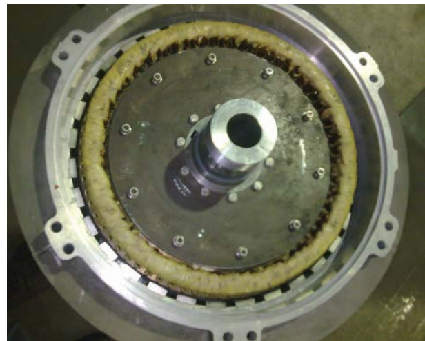
Fig. 11: Prototype generator with outer rotor.
