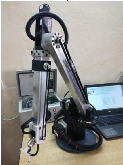
Figure (1): Three links robot manipulator 6 DOF
