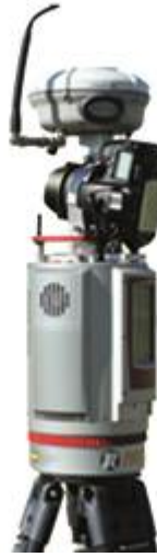
Figure 12. RIEGL VZ-400i with Nikon D810 and Trimble R8 GNSS-Receiver with RTK antenna.
