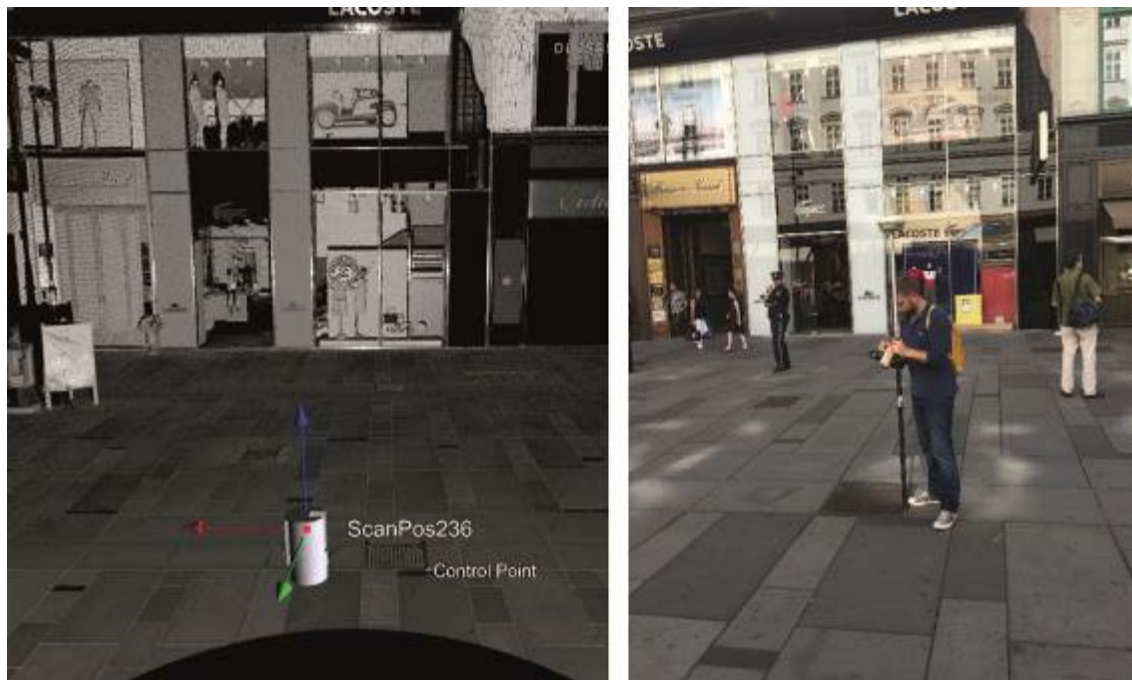
Figure 5. On the left: Data of scan position 236 including indicated control point. On the right: measuring of the control point of the same position using a Trimble R8 GNSS receiver.
