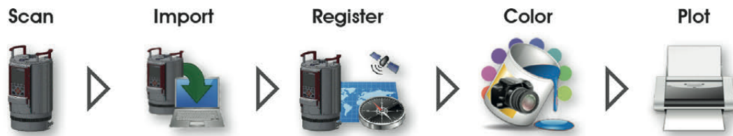
Figure 6. Schematic workflow of RiSOLVE (colorization was not applied in this project).
