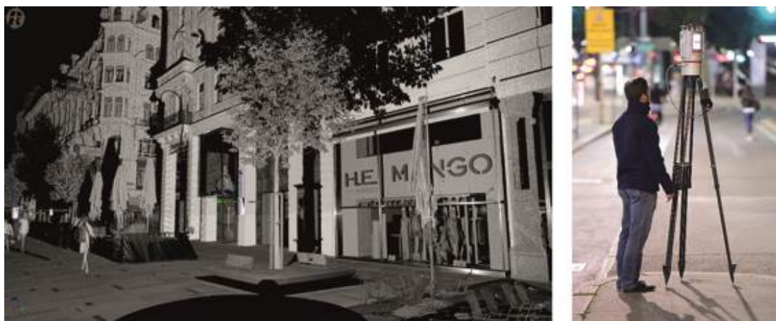
Figure 4. On the left: single scan ("Panorama 50"); the grey scale value represents the "reflectance". On the right: single operator with the RIEGL VZ-400i laser scanner.
