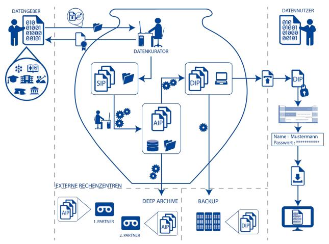
Figure. 2. Workflow of data submission, curation and dissemination according to the OAIS Model.
