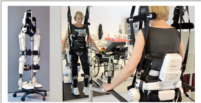
FIGURE 2 | HAL exoskeleton and training setting. Left part of the figure shows HAL exoskeleton with its electronic actuators for hip and knee joints (“power units”), its battery pack and controller at the top and its EMG-electrodes and cables for detection of bioelectrical signals. Right part of the figure demonstrates the training setting with the treadmill, the body-weight support and the exoskeleton. Official picture of Cyberdyne Inc., the person was not subject of the published study and has been engaged and paid for commercials. Copyright Cyberdyne, Inc., published with kindly permission.
