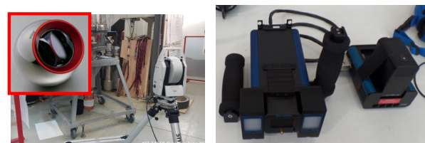
Fig. 6. Laser tracker (and its target), on the left. Camera used for the photogrammetry, on the right.
