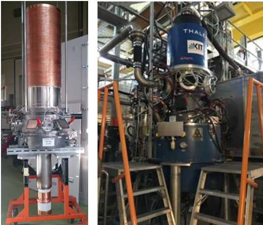
Fig. 1. TH1509 gyrotron prototype (left) and the same gyrotron installed in the KIT test stand (right), in Karlsruhe (Germany).
