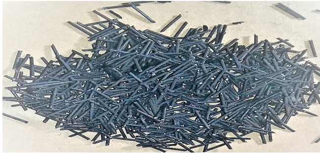
Fig. 1. Waste tire steel fibers of 10 mm length.
