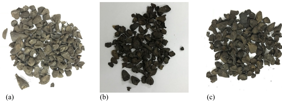
Fig. 2. Condition of oil palm shell (OPS), (a) before pre-treatment, (b) pre-treatment with common (26°C) water, (c) pre-treatment with hot water (50°C).
