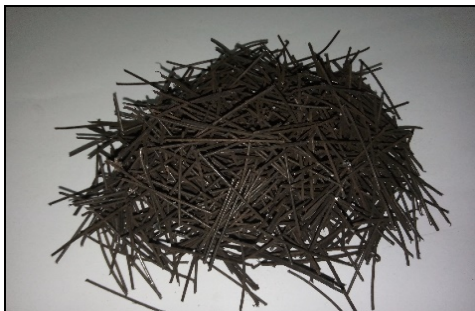
Fig. 3. The 4 cm length of steel fiber waste tyre.
