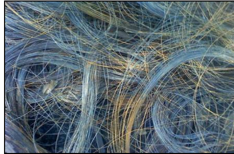
Fig. 2. Steel fibers extracted from waste tyre.
