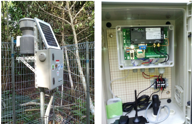
Fig. 4. The SESAME System for recording air temperature and rainfall data at Sungai Tohor Village.
