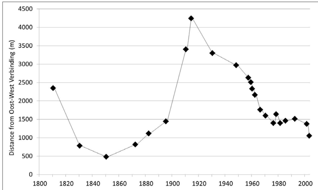
Figure 3: Erosion and accretion of shoreline near Totness, Coronie, from 1810 to 2003, relative to a fixed road called Oost-West Verbinding (modified from Augustinus and Teunissen 2004).
