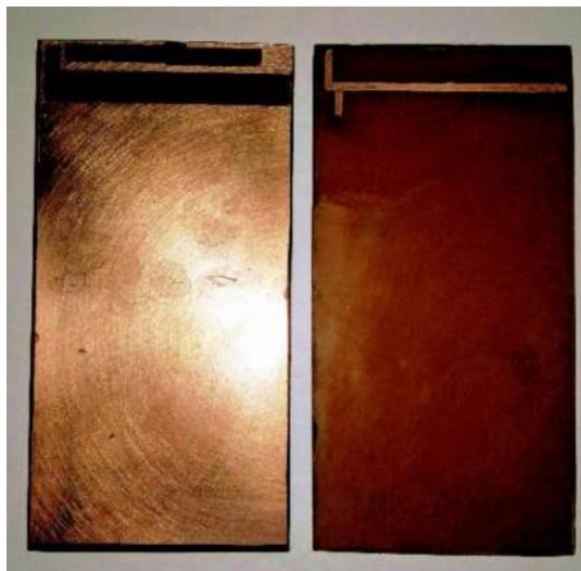
FIG. 10. PROPOSED GPS AND LTE BASED CELLULAR ANTENNA FABRICATED TOP AND BOTTOM LAYER PROTOTYPE
