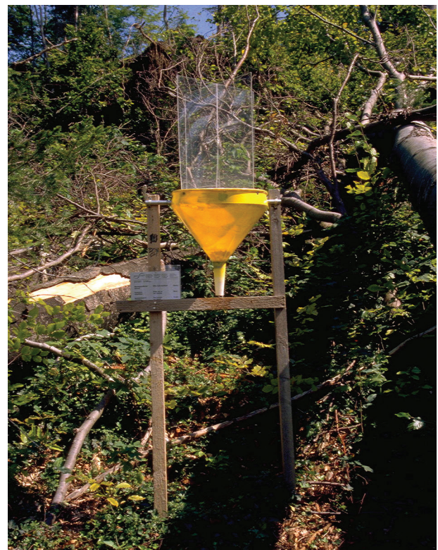
Figure 2. Combi trap (a combination of a flight interception trap and a yellow funnel trap) in an uncleared windthrow plot (Windthrow II) near Habsburg after storm Lothar. Photo: WSL.
