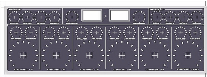
Figure 8 – Conceptual layout of operational controls and visual displays
