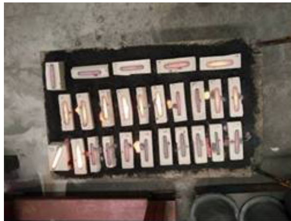
Figure 5 Casting process of samples in a mold (Tellurium powder is inserted into the mold before being cast)
