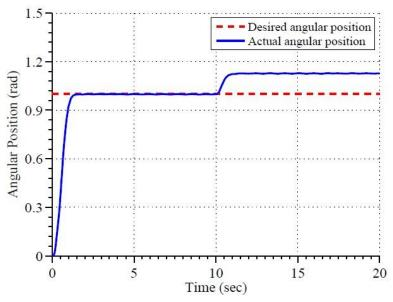
Figure 2. Desired trajectory tracking of the flexible joint manipulator by SMC law.
