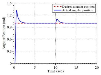
Figure 3. Desired trajectory tracking for flexible joint manipulator by integral SMC law.
