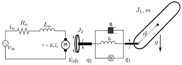
Figure 1. Block diagram of the flexible joint manipulator.
