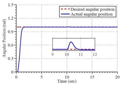
Figure 4. Desired trajectory tracking for flexible joint manipulator by DO based SMC law.
