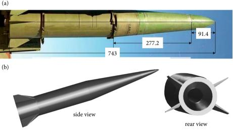
Figure 3. A PRAHV model of Kinzhal-like vehicle. (a) Iskander measured in photoshop (pixels); (b) 3D model of a PRAHV same size with Iskander
