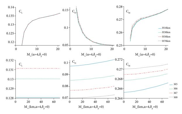
Figure 6. Relationship between aerodynamic coefficients and Mach number and height.
