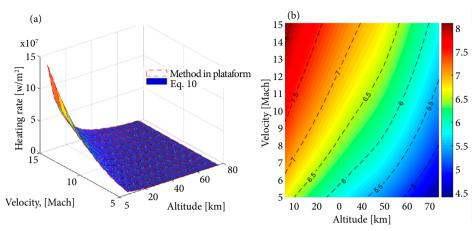
Figure 9. Heating rate of nose along the flight corridor of PRAHV.
