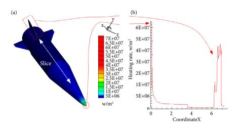
**Figure 8.** Aerothermodynamic environment ( $M_{\infty} = 10$ , H = 20 km,  $\alpha = 0$ ,  $\delta_p = 0$ ). (a) thermal environment over PRAHV surface; (b) heating rate on a slice along center line
