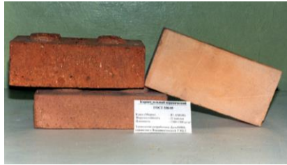
Fig. 5. Ceramic brick made from ASW of VCHPP-2 (ash enrichment 80%, M - 120÷150).
