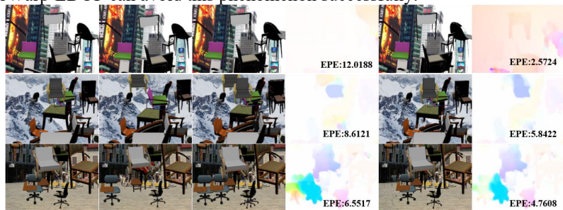
Fig. 4. Illustration of optical flow estimation on Flying Chairs dataset. In each row left to right: I_1 , I_2 , warped image based on the traditional method, optical flow estimation of LDOF, warped image based on our method, optical flow estimation of GrWarpLDOF. For all methods, the endpoint error is printed in the image.
