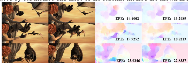
Fig. 5. Illustration of optical flow estimation on temple 3. In each row left to right: I_1 , I_2 , optical flow estimation of LDOF, optical flow estimation of GrWarp-LDOF. For all methods, the endpoint error is printed in the image.
