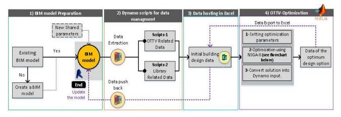
Fig. 2. Computational BIM-based OTTV-cost optimization model
