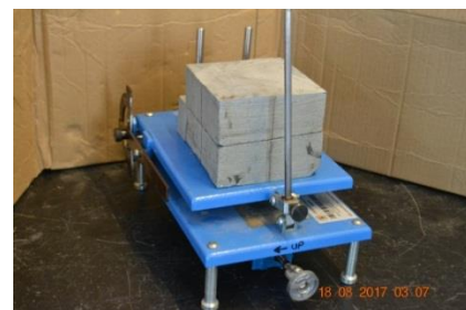
Figure 4: The tilt testing of square types samples.
