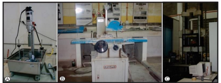
Figure 3: The coring machine, polishing and Hoek cell for triaxial test.
