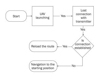
Figure 3 – Decision algorithm in case of signal loss between the UAV and the control station
