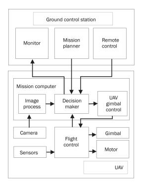
Figure 2 – Basic structure of the UAV's hardware system [23]
