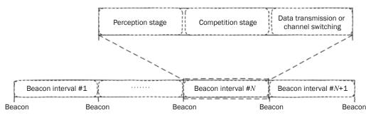
Figure 2 – Timing structure
