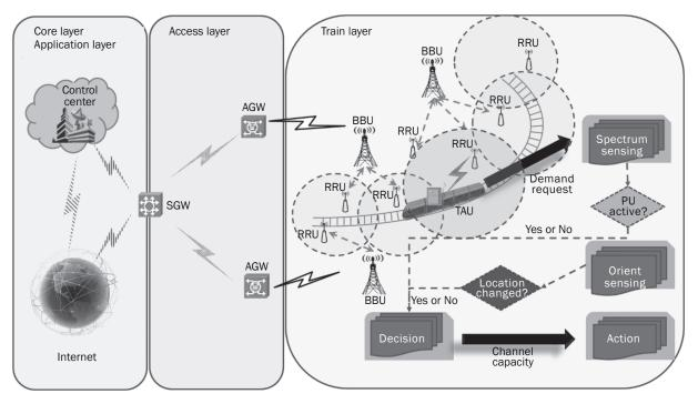
Figure 1 - Railway wireless communication network
