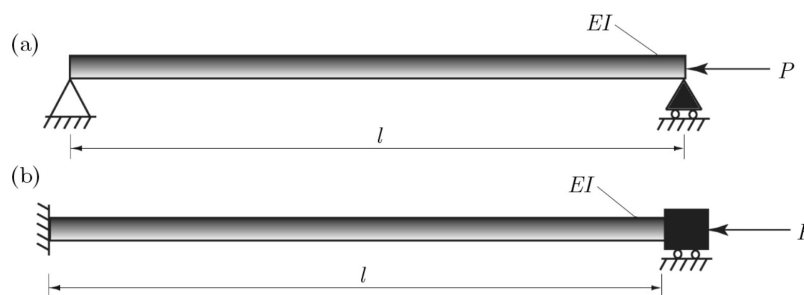
Fig. 1. Schematic of an Euler-Bernoulli beam subjected to an axial load (a) simply-supported beam, (b) clamped-clamped beam.
