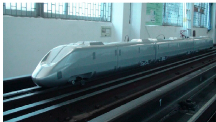
Fig. 16. The 1:16.8th scale model of EMU high-speed train [34].
