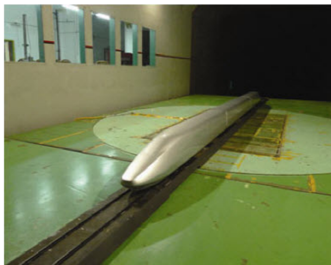
Fig. 8. The 1:8th scale model of high speed train [18].
