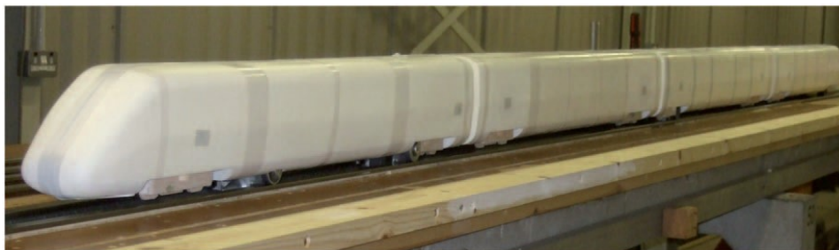
Fig. 9. The 1:25-scale of ICE2 German train (x = 4.216 m, length, y = 0.123 m, width, z = 0.156 m, height) [19].
