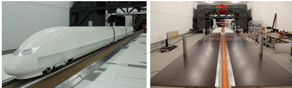
Fig. 12. The scale model of Germany high-speed train [23].
