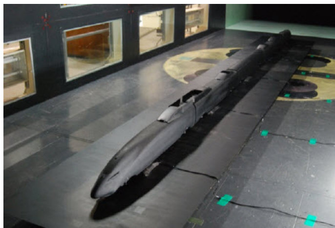
Fig. 12. The scale model of the Korean high-speed train [26].
