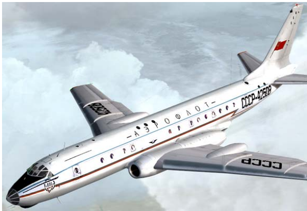
Fig. 6. One of the first in the world Soviet jet multi-passenger aircraft of the Tu-104 type («Russian camel» in the terminology of the NATO countries) developed by A.N. Tupolev (1956) based on a Tu-16 type combat aircraft [6]
