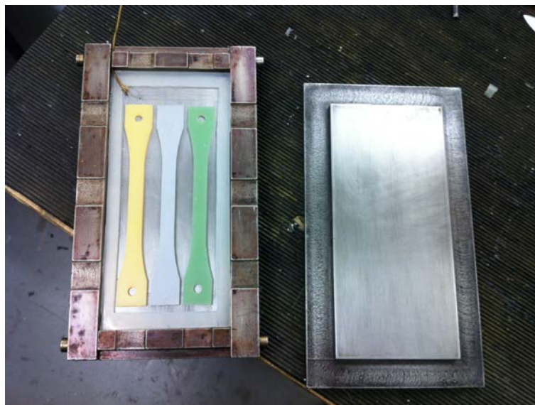
Figure 1: Mould with embedded thermocouple and sample specimens
