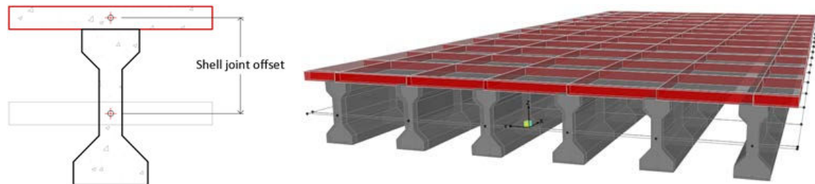
Figure 3: Slab and girders composite action
