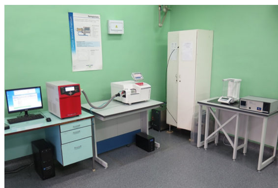
Fig. 3. The experimental complex for investigating the corrosion resistance of structural materials of NR and FR as a result of their interaction with various gases and gas-vapor mixtures.
