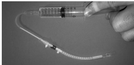
Fig. 9. Assembled catheter prototype being steered hydraulically. This is a PETG structure with a silicone skin of the same type as shown in Fig. 8.
