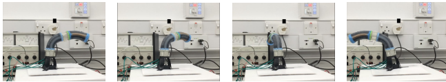
Fig. 8. The experiment shows the 2-segments soft continuum manipulator avoids a simulated plane obstacle (black) using magnetic-field-inspired navigation.
