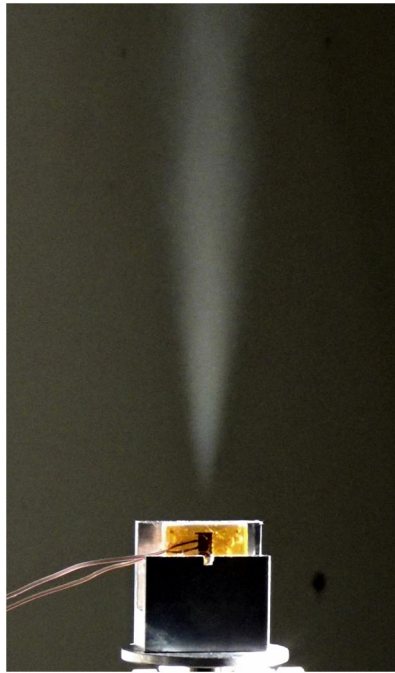
Fig. 6 Firing of the microthruster with cooling channels.
