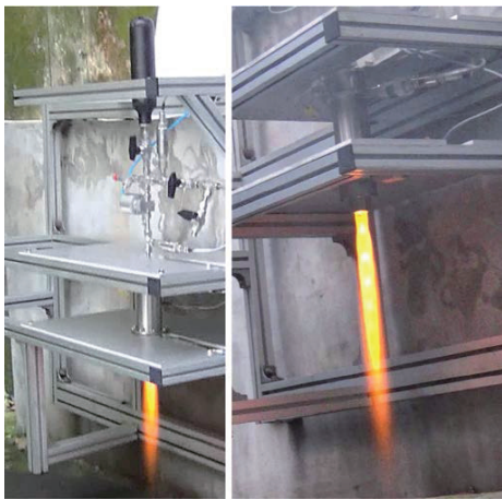
Fig. 4. Static combustion test of the hybrid rocket stand-alone system
