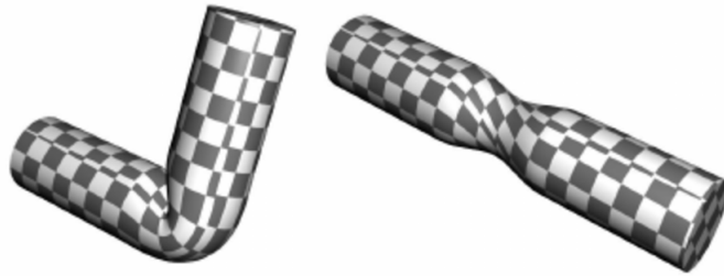
Figure 4.14: The loss of volume in the bent area and the “candy wrapper” effect when the joints are twisted.
