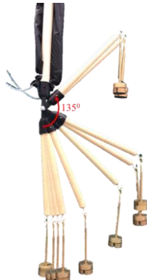
Figure 7. The agonistic movement of the arm. Angular displacement for the load of 3 N.
