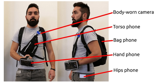
FIGURE 2. A participant wearing the four smartphones and a camera during data collection.
