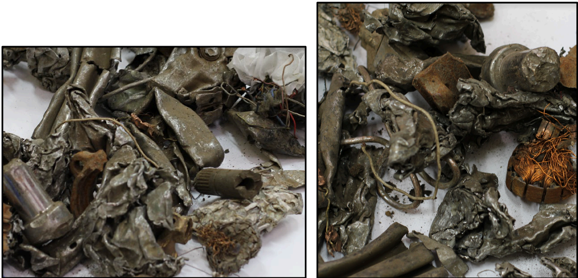
Figure 2.3: Images of copper wiring entangled in steel scrap obtained from a UK scrap yard.
