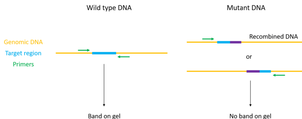
Figure 3.19: Scheme for relaxant screening of putative filipin recombinant strains. By using primer pairs that amplify across the target region, a wild type strain can be identified. A recombinant strain would not give a product. This method is obviously not a reliable way to confirm a recombinant strain but provided a starting point for further confirmation.
