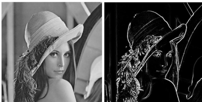
Figure 2.6: The power of the convolutional operator, demonstrated on the Lena image used for computer vision benchmarking. With a very small amount of parameters (e.g. 3 \times 3 kernel matrices), convolutions are capable of extracting valuable information such as edges out of an image (which often encode most of the valuable information therein).
