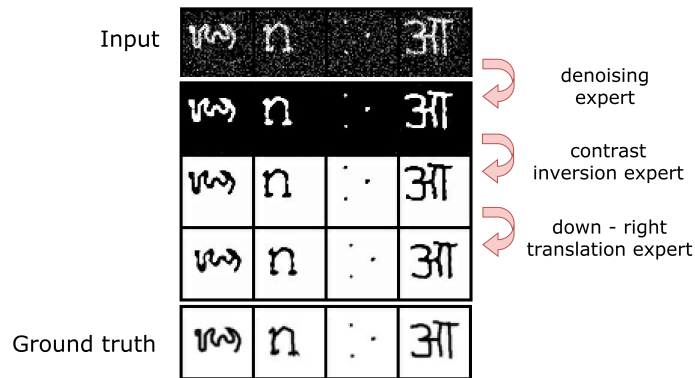
Fig. 3.17 First row: Omniglot letters that were transformed by a combination of transformations (noise, contrast inversion and translation up left). Second to fourth row: application of denoising, contrast inverting and right down translating experts. Last row: ground truth. Although the experts were not trained on a combination of mechanisms nor on Omniglot letters, they can be used to recover the original symbols.
