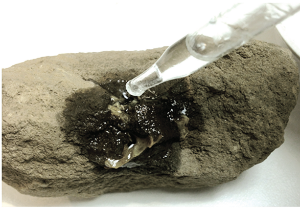
Figure 3 Application of CDD to a heated block of porous matrix and fragile specimen. CDD easily wicks into the specimen, filling pore spaces and voids. Photo: G. Brown.
