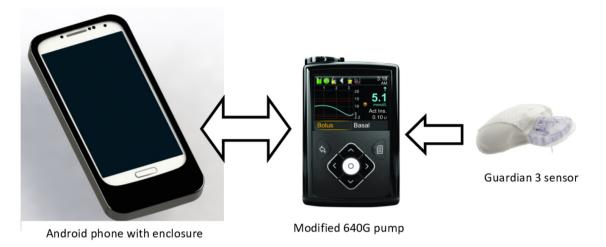
**Figure 2** FlorenceM closed-loop system prototype. The system consists of a continuous glucose monitoring transmitter with Guardian 3 sensor (Medtronic), an insulin pump (modified 640G pump, Medtronic) and an Android smartphone running the control algorithm (Cambridge).
