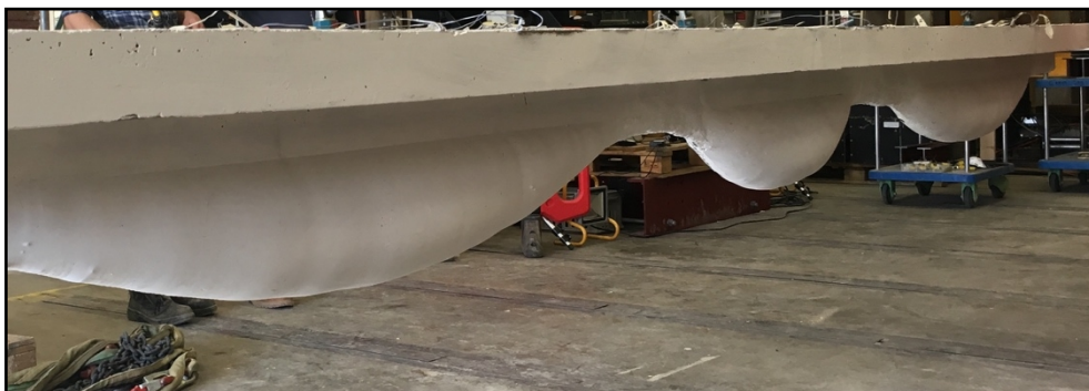
Figure 2: Fabric-formed continuous concrete beam cast at the University of Bath (credit Tayfur, 2016)
