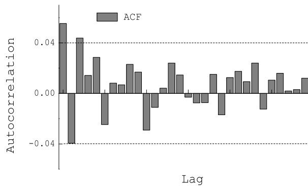
Figure 7.b. Correlogram of the (Z - \text{mean}(Z)) series calculated with one-step ahead predictions from the MS(2) - AR(3) model obtained via rolling regression over the testing wind speed time series.
